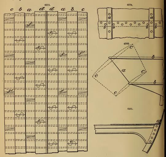
Have the inside strakes stitched at the butt-straps and frames, say about six rivets in each buttstrap and two in each frame, before putting on the outside strakes. The filing-plates at the bulkheads at back of shell-plates should be at least the width of
